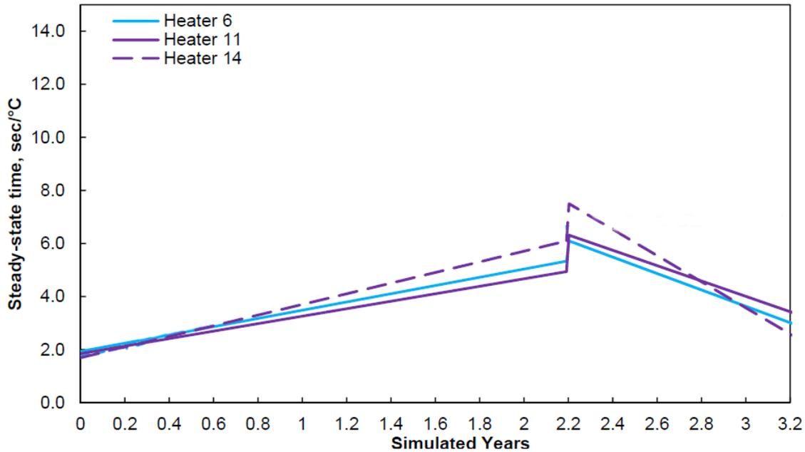
Figure 7. Phase II heaters with a decrease of time to steady state.
