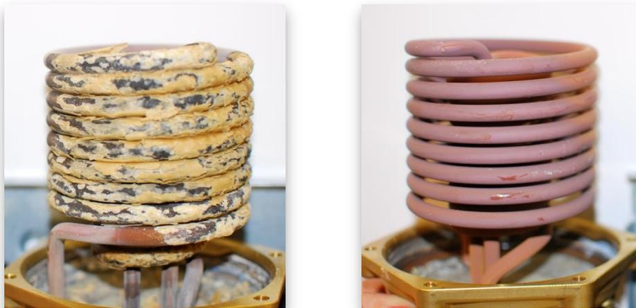
Figure 3. Untreated Element (Left) and Treated Elements (Right)
