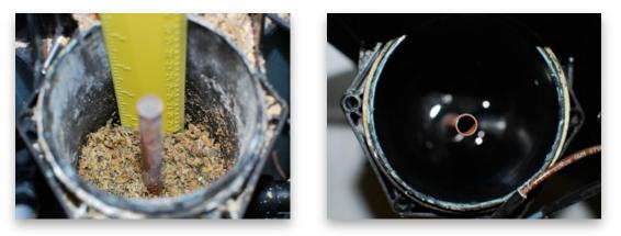
Figure 4. Untreated Canister (Left) and Treated Canister (Right)
